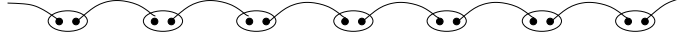
Figure 1: The AKLT state is constructed by considering each spin-1 site as consisting of two spin-1/2 parts that are symmetrized. In each site, one part forms a singlet (solid line) to its right, and the other part forms a singlet to its left. Parameterizing the spin-1/2 parts using Schwinger Bosons enforces their symmetrization.
